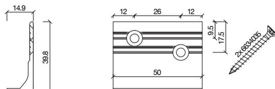
4451540 Equerre de fixation antichute 40x15x50 mm FV/FVNG
